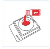
Open the pouch of the membrane unit without touching the test window. Immediately after, pour Solution 1 with the specimen into the center of the membrane unit test window. Solution 1 has to be poured into the test window within 5 minutes of adding the sample. Allow to absorb completely.
