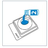
Mix Solution 2 thoroughly by slowly inverting the bottle. Pour Solution 2 into the center of the test window. Allow to absorb completely.
